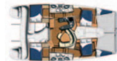
The Moorings 4300 version, with four double cabins and accommodation in the two forepeaks.
