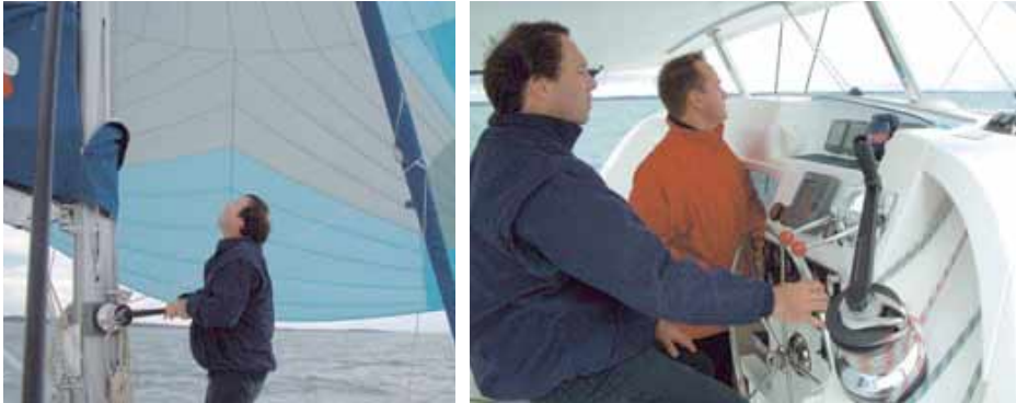
ABOVE, LEFT: With a 6m beam, a spinnaker pole is superfluous. RIGHT: The cockpit layout allows for most tasks to be controlled from the helmsman's seat
